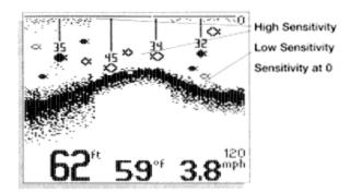
Increasing the bias (+1 through +5) causes the unit to display the information from progressively smaller sonar returns. By decreasing the sensitivity bias (-1 through -5), the unit effectively filters small sonar returns.
